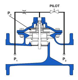
P<sub>1</sub>: Inlet pressure/upstream pressure
