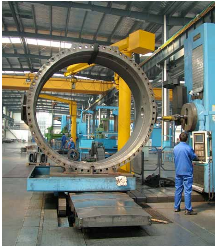
Series 756 DN 2800 - Body machining at AVK ANHUI.
