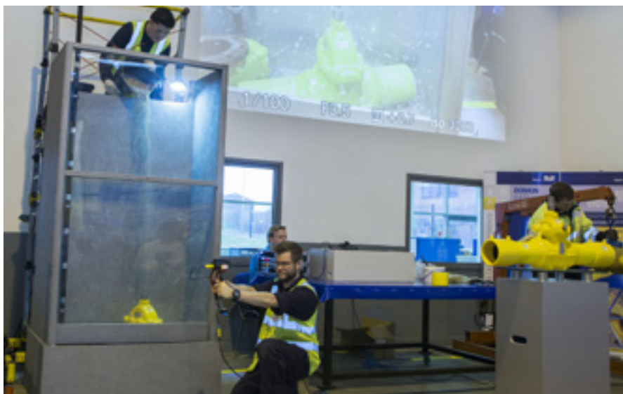
Chip test with 32 kg of aggregate dropped from 2 meters
