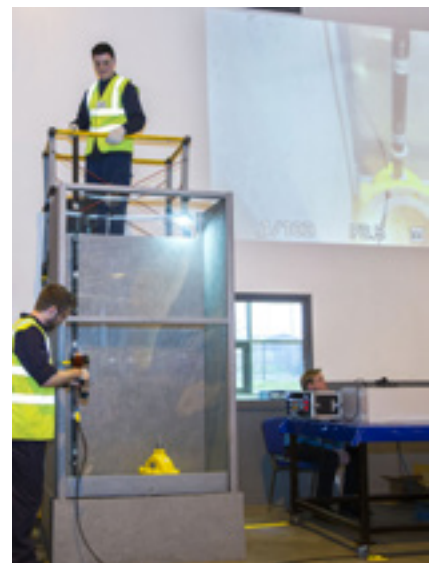
Impact test dropped from 1.5 meters
