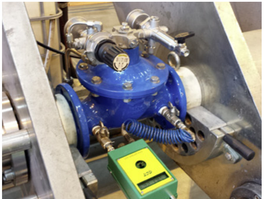
S859 PRV and data logger on test rig at BDV
